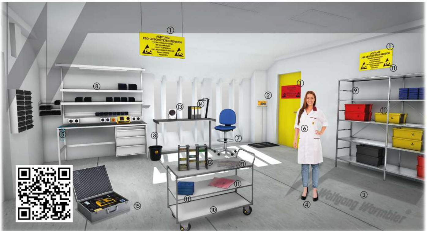
ESD protected area (sample configuration)
